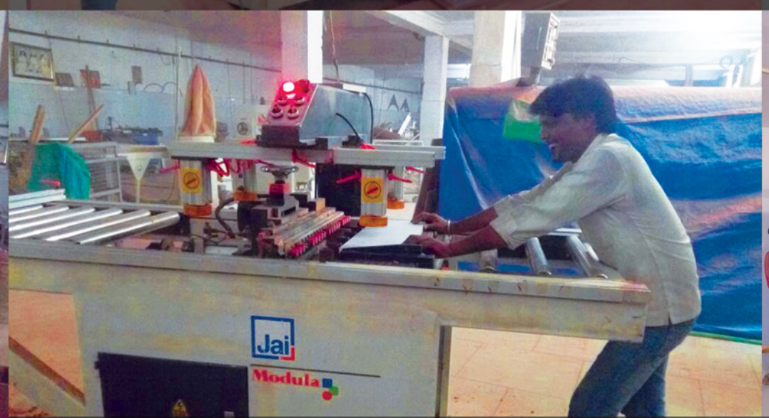
MULTI-BORING MACHINES In this process, all the boxed cabinets are attached by concealed screws, imparting a modular finish.
