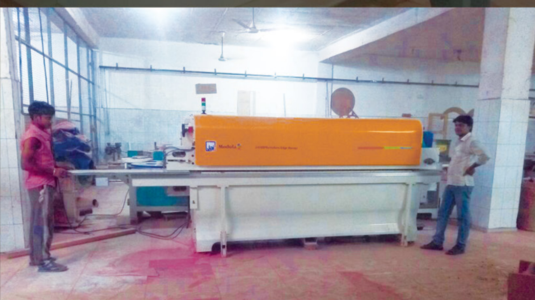
TROUGH-FIT MACHINES In this process, the board is beaded till 250 degree celsius temperature to give it a permanent fixture.
