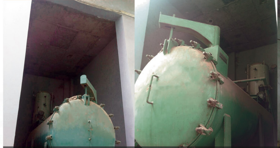
ANTI-TERMITE PLANT Wood is made termite-resistant by injecting chemicals, to enhance its life.
