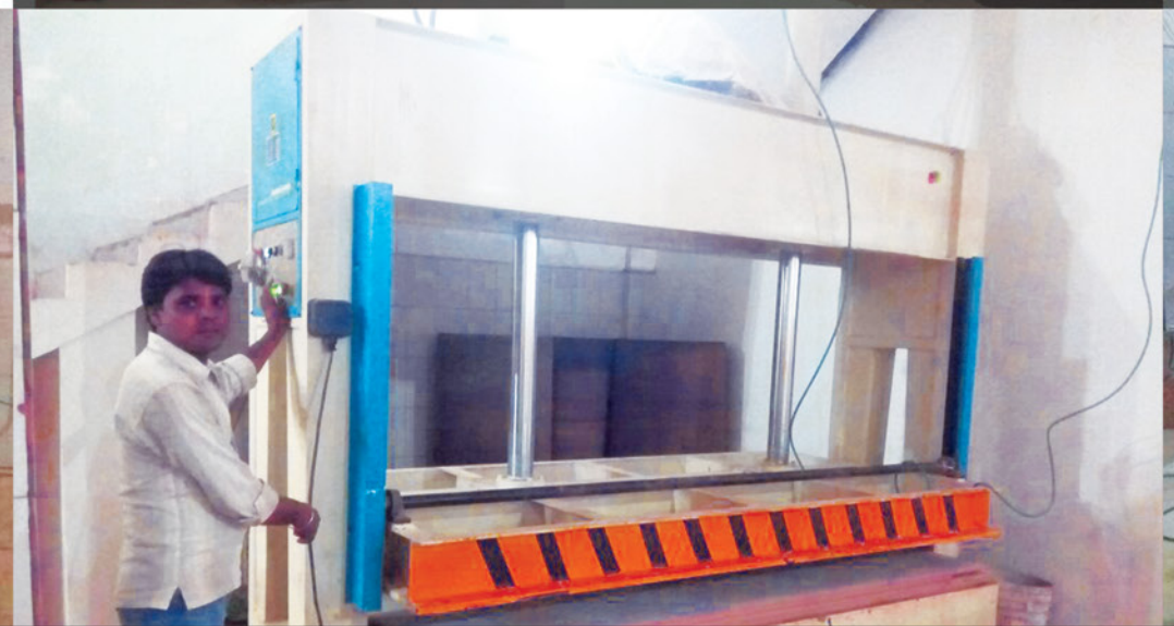
50-TON COLD PRESS All the laminates are pasted mechanically to avoid air bubbles over block boards.
