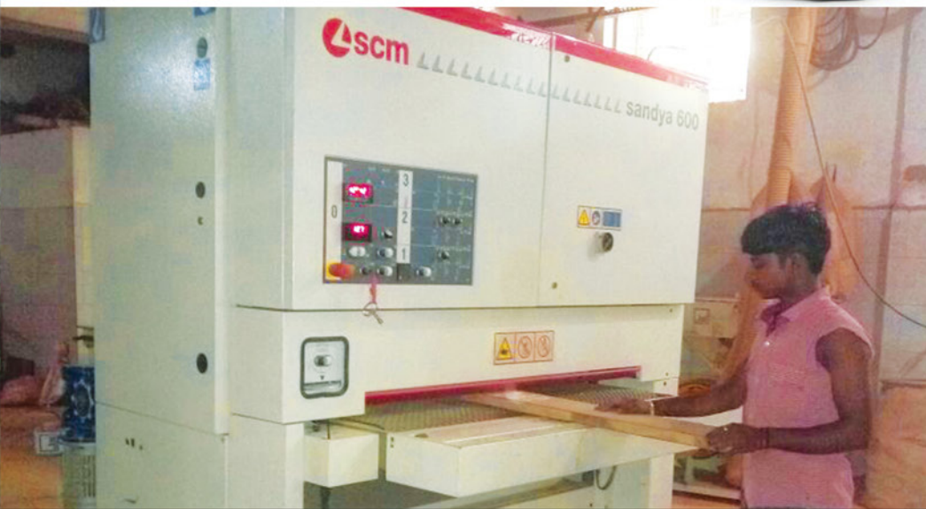
SANDING MACHINES In this, wood is rubbed through the series of embri belts, to make the ends smooth.
