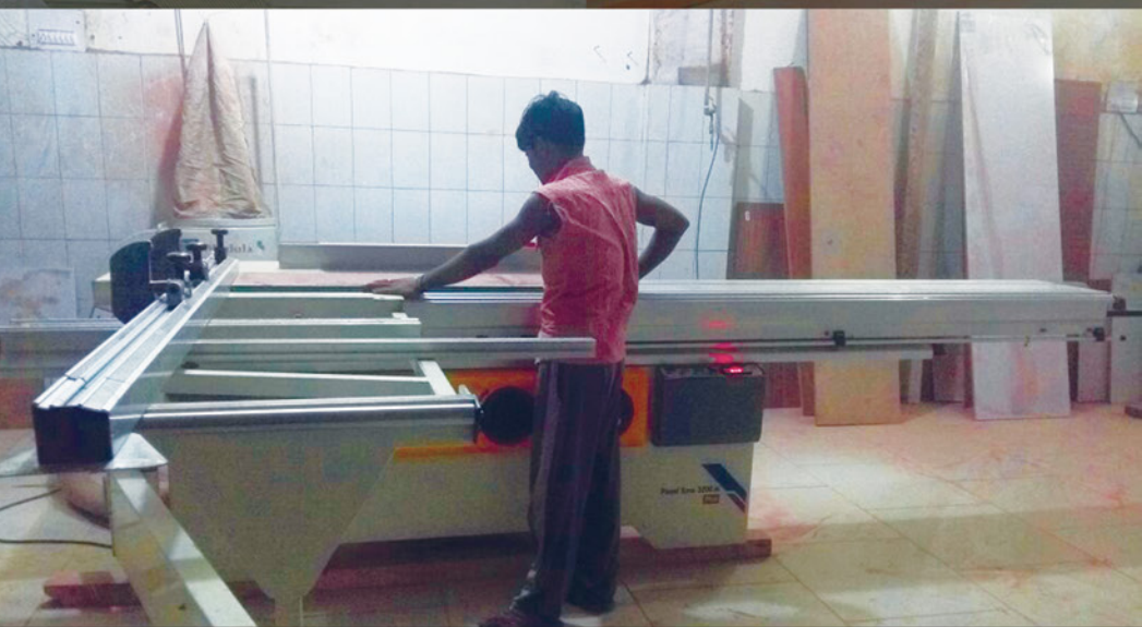
PANEL SAW Cuts the board and wood to ultimate fineness and produces joint-less cuttings.
