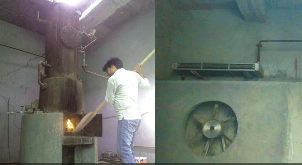
SEASONING PLANT In chamber, wood is seasoned to reduce its natural moisture, to make it retain its shape and lusture forever.
